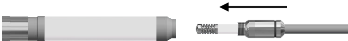
Figure 5: Igniter installation into Base Rod.
